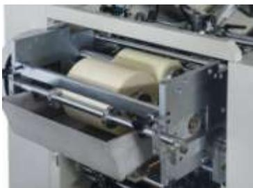
**The compact design of mechanical transmission**
