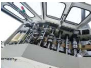
**monolithic cylinder-forming adjusting structure**
