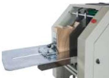
**Bag Bottom Gluing Structure**
